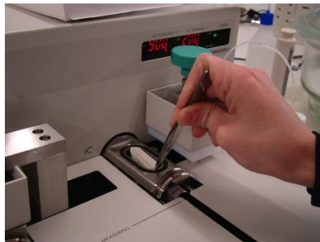
Photo 13: Placing the ceramic boat into the TOC-VcsnShimadzu (Source: Šmid, 2011)
