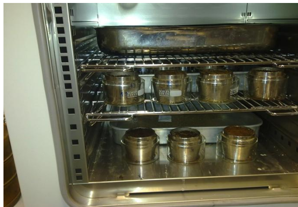
Photo 9: Drying the water saturated samples in the ventilated oven at 105°C (Source: Šmid, 2011)
