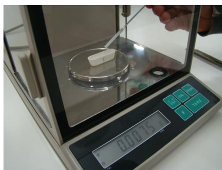
Photo 12: Measuring the amount of soil sample (Source: Šmid, 2011)
