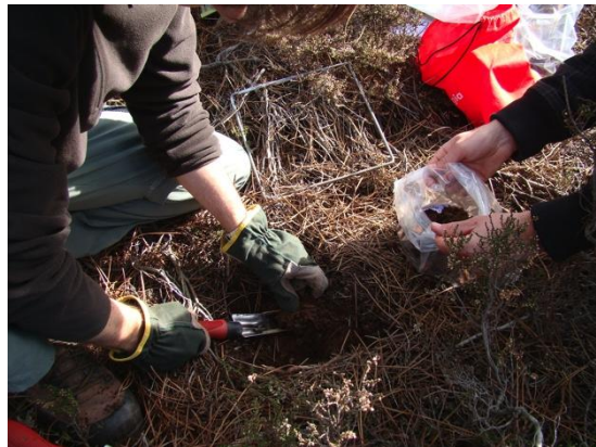
Photo 5: Taking the soil samples before fire (Source: Šmid, 2011)
