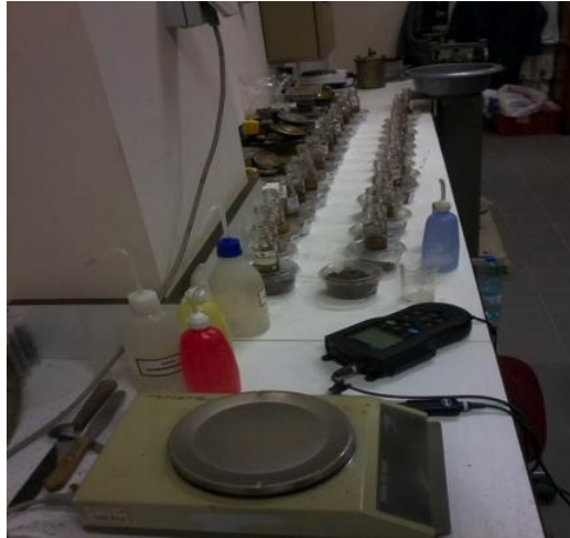
Photo 10: Sample preparation for determination of soil pH and soil electric conductivity (Source: Šmid, 2011)
