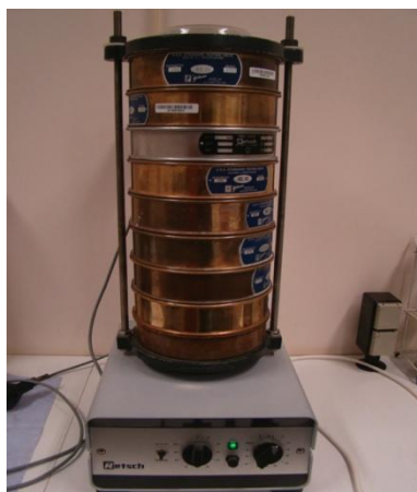
Photo 8: Preparation of laboratory samples with sieving vibrator device (Source: Šmid, 2011)
