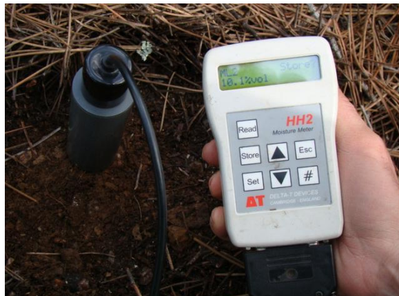
Photo 6: Measuring the soil moisture (Source: Šmid, 2011)
