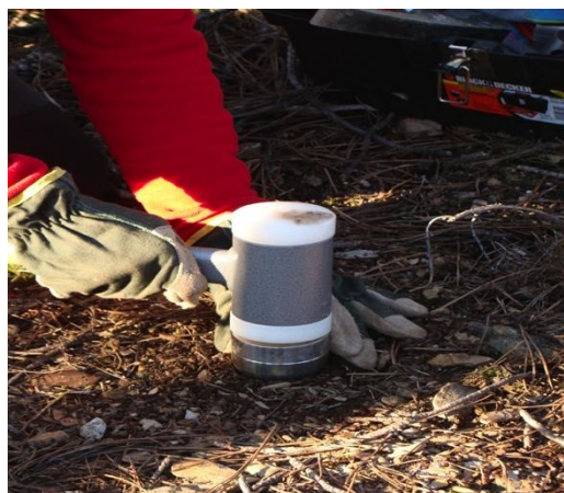
Photo 7: Taking the cylinders samples for determination of soil bulk density (Source: Šmid, 2011)
